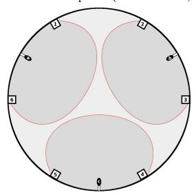
Each microphone covers roughly one third of the location area. Each sound produced within the sector of a microphone should be captured by that microphone at a higher level than by the others. The microphones should be installed at the same height than the speakers, and the angle must be carefully registered in order to get as close as possible to the above scheme.
